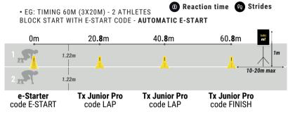
To trigger the start procedure: press the button at the top of your e-Starter > et ready at the SET sound > take the start at the BANG sound
