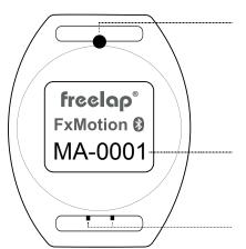
**Led:** Indicates that the device is waking up / gives the battery level.
