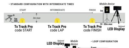
Place your mobile device from 10m to 50m maximum after the FINISH transmitter, at a height of approximately 1m from the ground.
