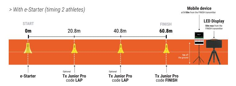
e-Starter transmitter can cover 2 lanes. Place it between the 2 lanes.
