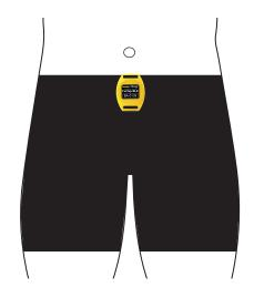
Attach your FxChip BLE to the athlete using his attachment clip (provided): Insert the clip into the notch at the top of the back of your FxChip BLE. Then hang the clip on the belt of the athlete's short.
