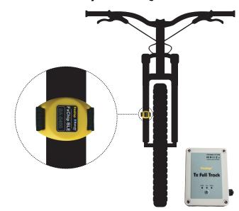
/!\ Attaching the transponder to any other location or position may result in inaccuracies or non-detection.
