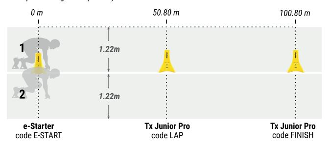
• When doing a block start, then you must place the next transmitters (code LAP and FINISH) **80cm after the desired distance**; because the chip will detect the transmitters 80cm before its exact position.
