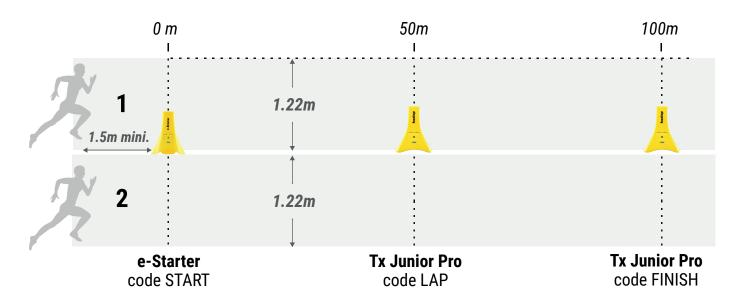
• In case of flying start, you should start to run at least 1.5m before the START transmitter to avoid early detection.
